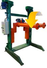
The rollers on which the tyre is positioned are driven electrically.
