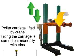
The rollers on which the tyre is positioned are driven electrically.
